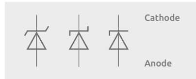
Figure 39 | Common symbols for a Zener diode.
