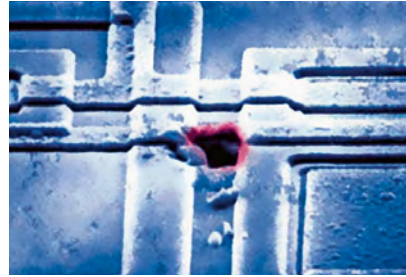
Figure 64 | Example of ESD damage
