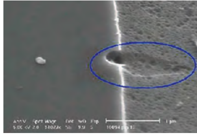
Figure 63 | ESD damage with small burn mark
